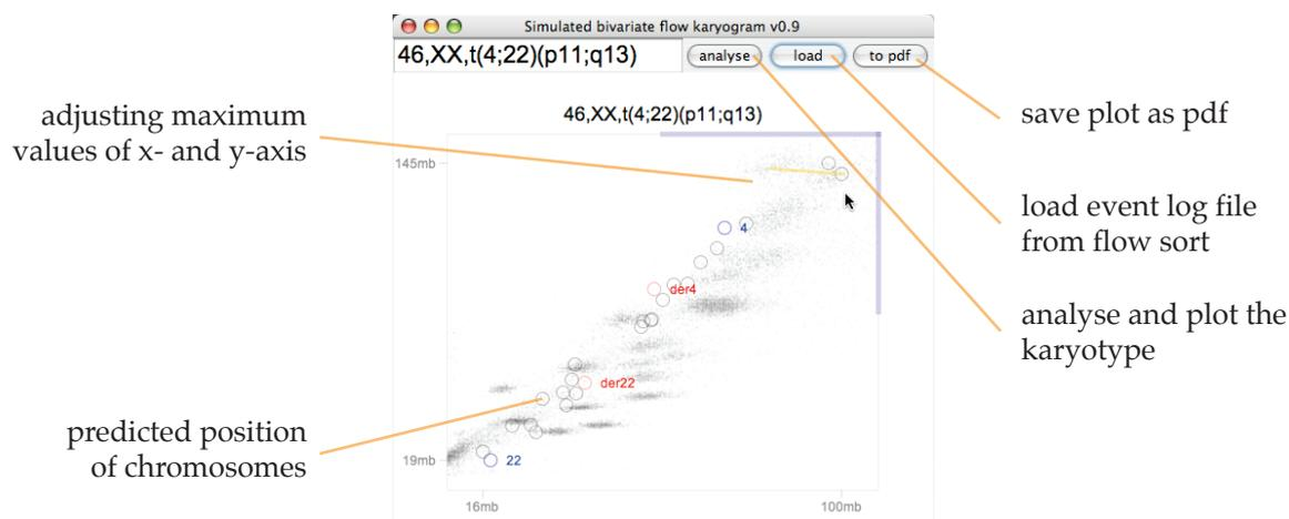
The event log values will most likely not fit the predicted values perfectly, therefore it is possible to adjust the axis by dragging the data. By dragging from different areas of the plot you can adjust minimum and maximum of each axis. When dragging the ends of the axis being adjusted will be highlighted.
